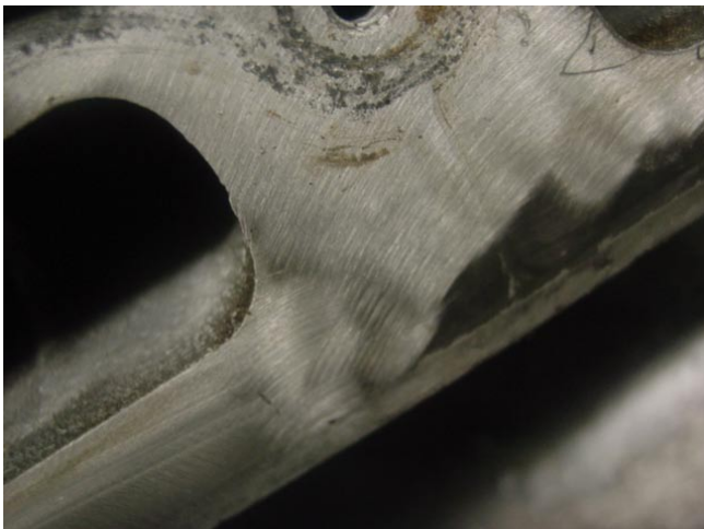
Fig 1 Note the brushed-looking surface from using a surface conditioning disc. The action releases aluminum oxide as well as metal particles removed from the base metal.
