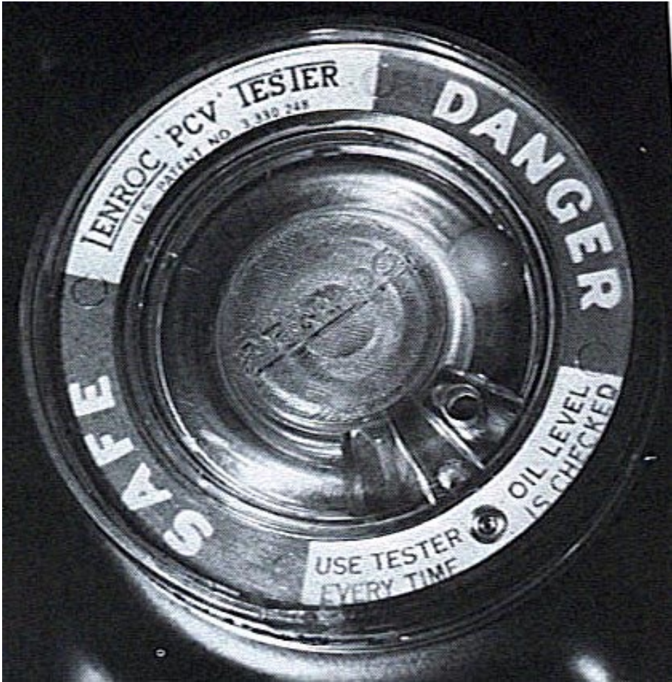
Figure 3 PCV flow tester that has a gauge built into unit that mounts in the filler cap position
